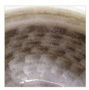
These are clearly recognizable in the photos of the polyamide grinding bowls, where 7-8 different levels of horizontal roll-off paths are seen, which already develop at the bottom radius and end below the grinding bowl lid. Incidentally is the deepest grinding path found here, since the grinding balls striking the grinding bowl lid always strike the upper area of the grinding bowl walls and roll off - due to the high centrifugal powers.
