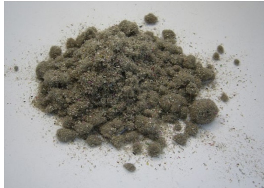
Fig. 5: after comminution – 0.5 mm sieve
