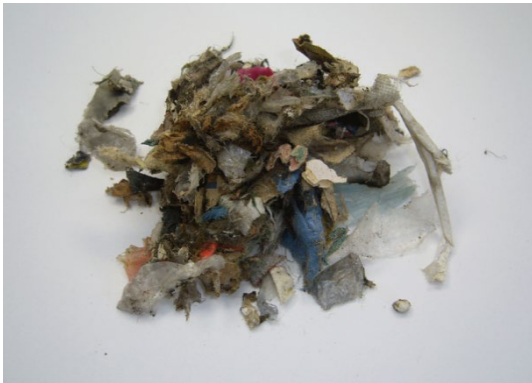
Fig. 4: Secondary fuel prior to comminution
