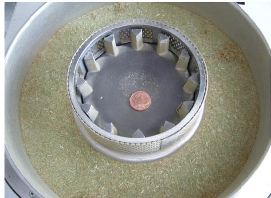
Fig. 4: Impact bar and 1 mm sieve
