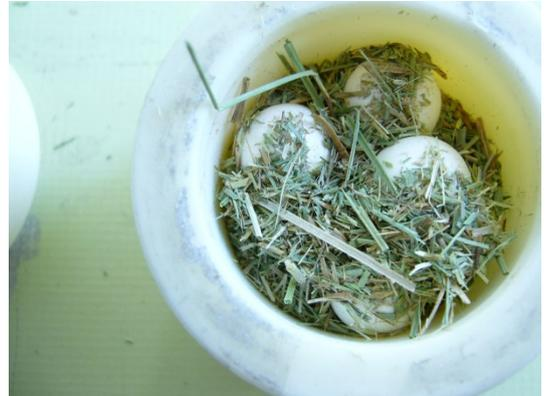
Fig. 7: Purple Moor-Grass in a grinding set made of sintered corundum
